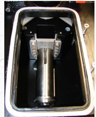
A Test Cell Attached to the Rotor
